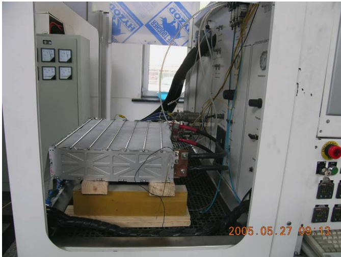
Fig. 8. The 10 kW (130-cell) stack using the expanded graphite bipolar plates. Active area was 270 \text{ cm}^2 .
